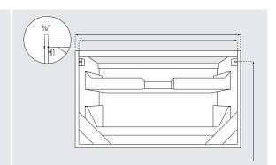
2. Separate the two hanging brackets by bending and cracking apart the included hardware. Drill mounting holes in wall and fasten wall brackets with screws.
