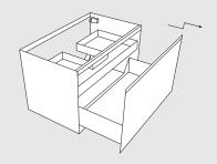
4. Hook vanity onto wall brackets. Mount support bracket onto wall directly under vanity base.
