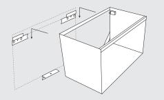
Adjust metal hooks if necessary to properly level vanity and secure it to wall.
