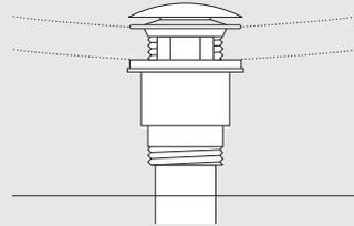
6. Fill tub with water until the overflow and then drain the tub. Maintain access below floor level and inspect the waste connections for leaks as the water drains.
