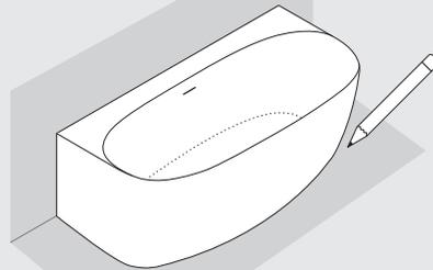
2. Move tub away, carefully placing it upside down on a protective surface. Measure distance from edge to drain pipe and mark location on floor.
