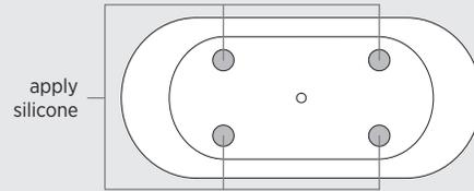
5. Carefully set tub into its proper position and connect drain fittings to tailpiece.
