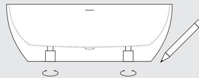
2. Move tub away, carefully placing it upside down on a protective surface. Measure distance from edge to drain pipe and mark location on floor.
