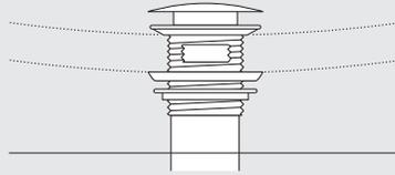
6. Fill tub with water until the overflow and then drain the tub. Maintain access below floor level and inspect the waste connections for leaks as the water drains.
