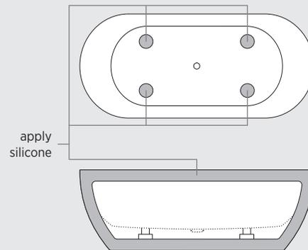
7. Carefully set tub into its proper position and connect drain fittings to tailpiece.
