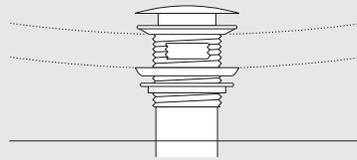
8. Fill tub with water until the overflow and then drain the tub. Maintain access below floor level and inspect the waste connections for leaks as the water drains.
