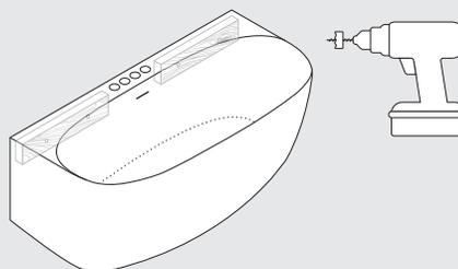
7. Generously apply adhesive or silicone to bottom of feet and top of wood block on wall.
