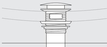
9. Fill tub with water until the overflow and then drain the tub. Maintain access below floor level and inspect the waste connections for leaks as the water drains.
