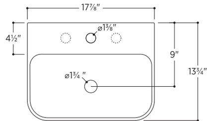
All measurements are approximate and for comparison only. Please note that these dimensions and specifications are subject to change without notice. Our products must be installed by certified professionals only and according to our installation guide, as well as federal, provincial/state and local building codes and regulations.
